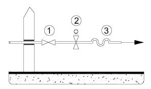
The gas system must be realized in compliance with the rules in force. Respect dimension of the dryer gas-connection written in the technical data sheet; this dimension must not be reduced.
