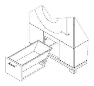
In both cases, the fluff must be removed from the filter using hands, do not use sharpened object.
