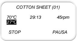
The final part of the program is a not heated cycle (cooling step) to ensure the linen will not be damaged.
